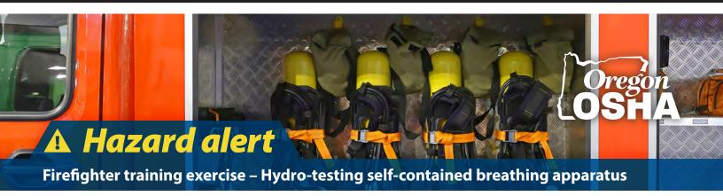
Residual nitrogen in a self-contained breathing apparatus (SCBA) cylinder after hydro-testing can dilute oxygen to dangerously low levels. If bottles are filled after testing without being purged, an air-monitoring device may show a full level of air, but the concentration of oxygen is weak enough to cause hypoxic effects or other respiratory trauma.
