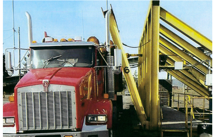
Secure loads by making contact with the adjustable barrier.
