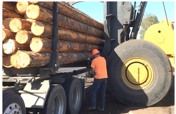
Secure loads by fully encompassing them with the grapple, and with the carriage backrest against the load.
