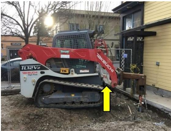
Takeuchi TL12V2 skid steer with helical attachment. Arrow Points to the spot where the victim was pinned between the lift arms' cross member and the cab.
