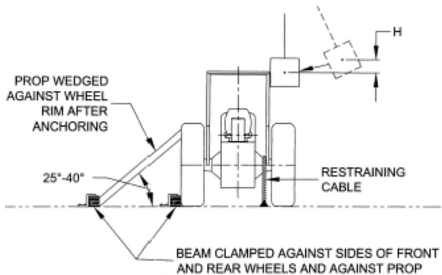
FIGURE W-23 - METHOD OF IMPACT FROM SIDE.
