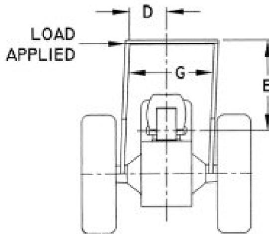
FIGURE W-16 - SIDE LOAD APPLICATION.
