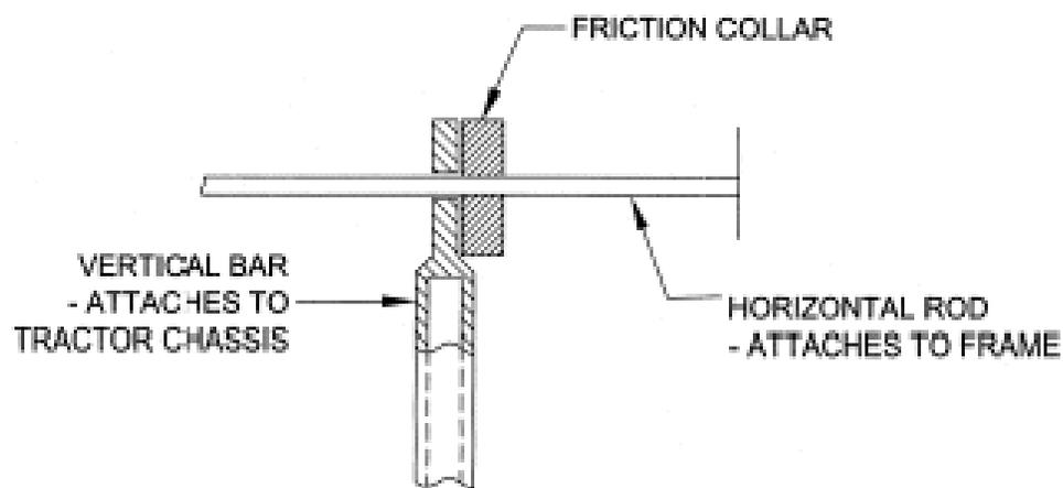
FIGURE W-18 - METHOD OF MEASURING INSTANTANEOUS DEFLECTION.
