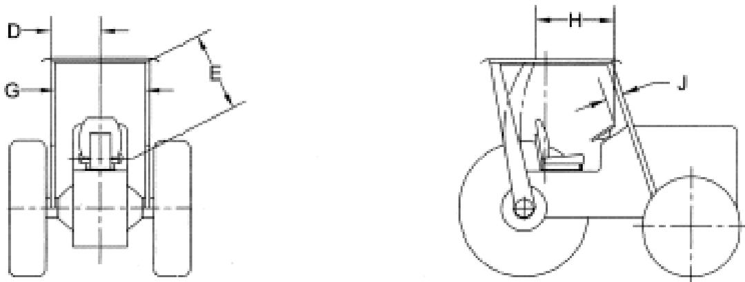
FIGURE W-28 - PROTECTED ZONE DURING CRUSH AND DROP TEST.
