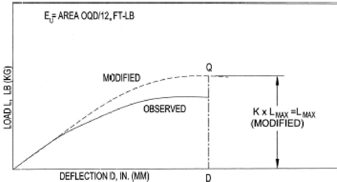
FIGURE W-20 - TYPICAL MODIFIED  $L_M$ - $D_M$  DIAGRAM.
