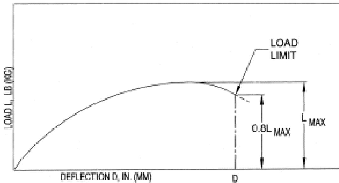
FIGURE W-19 - TYPICAL L-D DIAGRAM.
