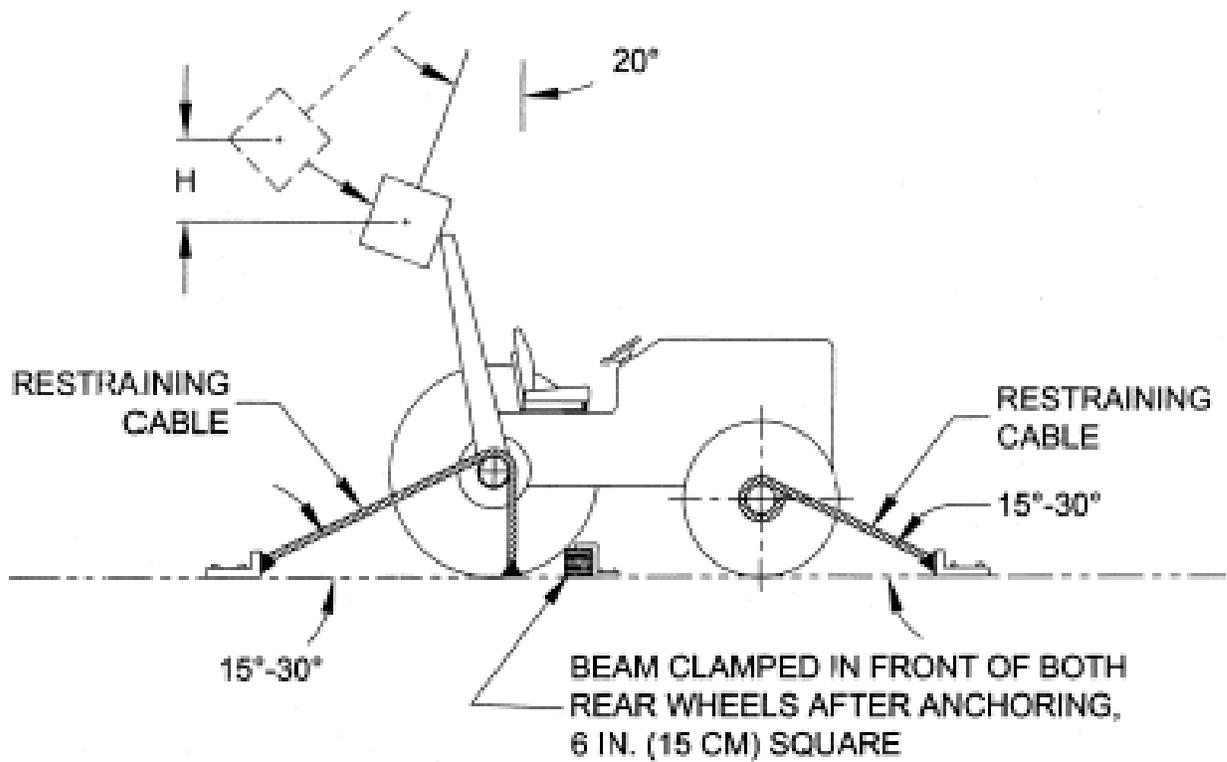
FIGURE W-22 - METHOD OF IMPACT FROM REAR.
