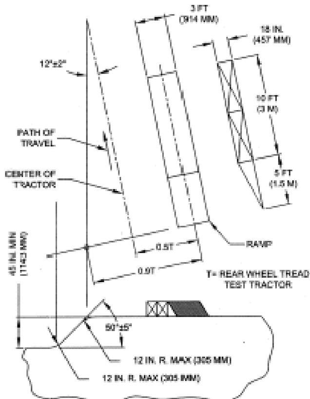
FIGURE W-15 - SIDE OVERTURN BANK AND RAMP.
