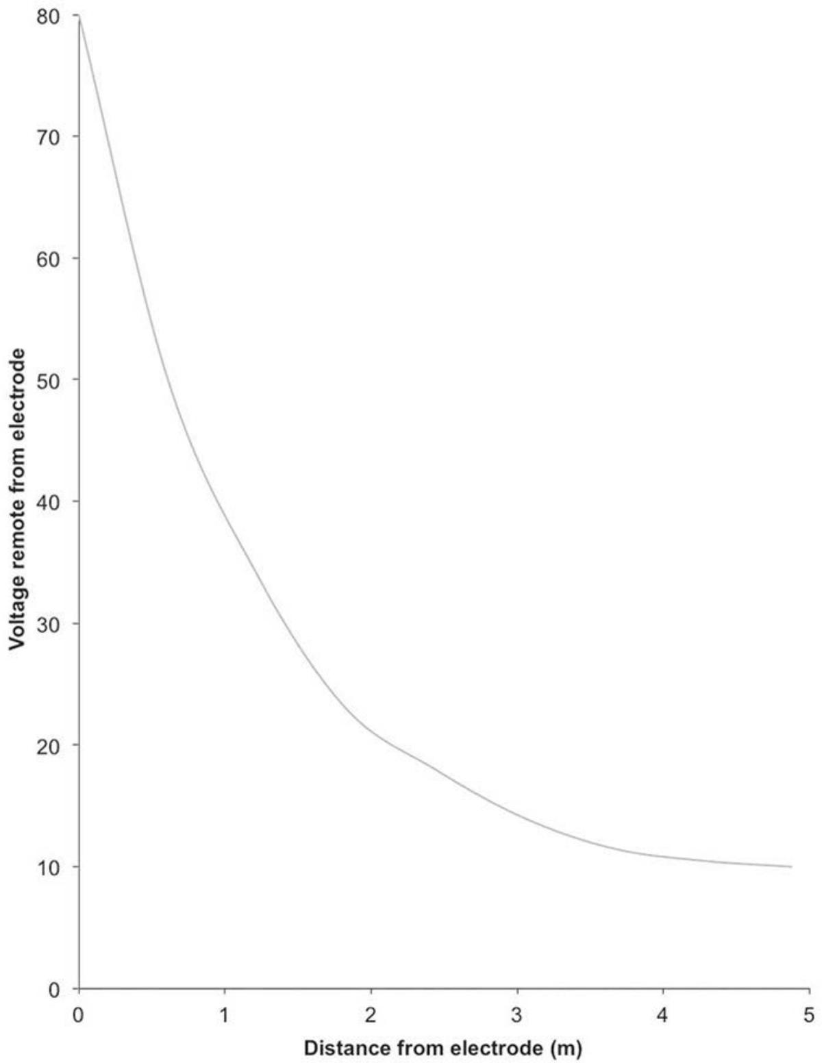
Figure 1 - Typical Voltage - Gradient Distribution Curve
