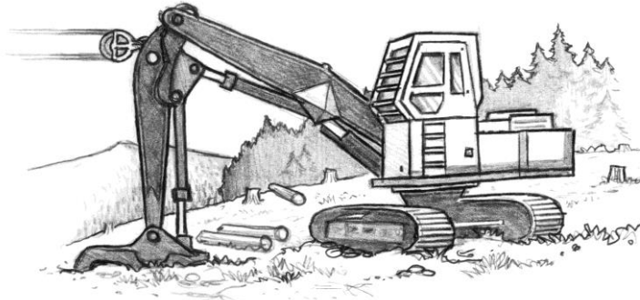
Figure 7-25 – Log Loader Anchor
