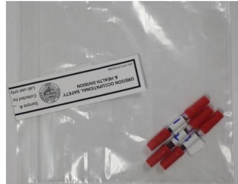
Charcoal tubes inside of a Whirl-Pak® with bag opening securely closed and sealed. Other media types, such as filter cassettes and bulk solid material (e.g. paint chips), may be sealed in this manner.
