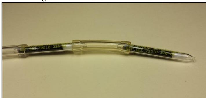
Figure 4. **SKC Dual Adjustable Low Flow Tube Holder for Sampling in Parallel**
