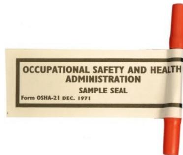
End caps can be removed, allowing sample integrity to be jeopardized without disturbing the seal
