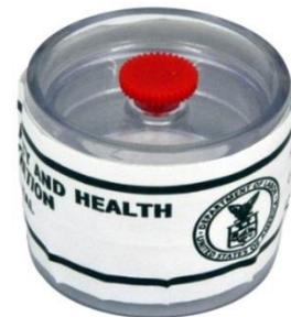
Lab seal covers inlet/outlet ports maintaining sample integrity.
