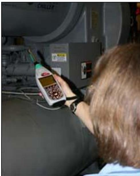
Confirm that the sound level meter is properly calibrated and temperature-stabilized. Then, position the microphone in the monitored worker's hearing zone. Oregon OSHA defines the hearing zone as a 2-foot-wide sphere surrounding the head. Considerations of practicality and safety will dictate the actual microphone placement at each survey location. Note that when noise levels at a worker's two ears are different, the higher level must be sampled for compliance determinations.
