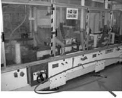
Seal off all small gaps and openings along all polycarbonate panel edges and the adjacent framework, and the bottom edge of the machine cabinet to the floor.
