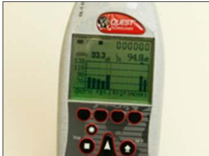
Some octave band analyzers can be set to automatic function (i.e., the instrument automatically checks the sound level of each frequency band and stores the results). Other instruments require the user to manually switch between the different frequency bands, recording each reading in sequence.
