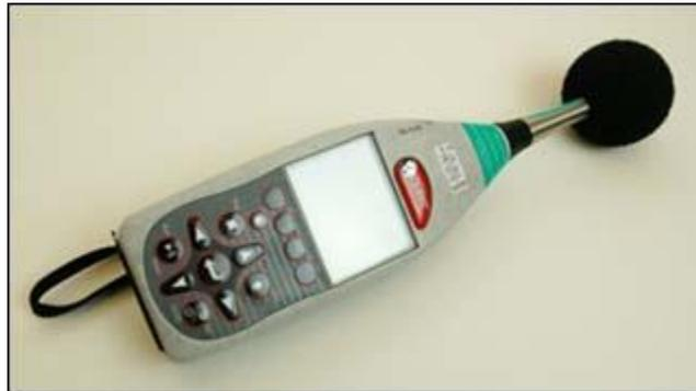
Most Type 1 and Type 2 sound level meters can be set to respond with either a "slow response" or a "fast response." The meter dynamics are such that the meter will reach 63% of the final steady-state reading within one time constant:
