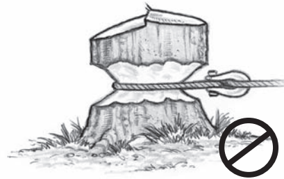
Improper notching: too deep
