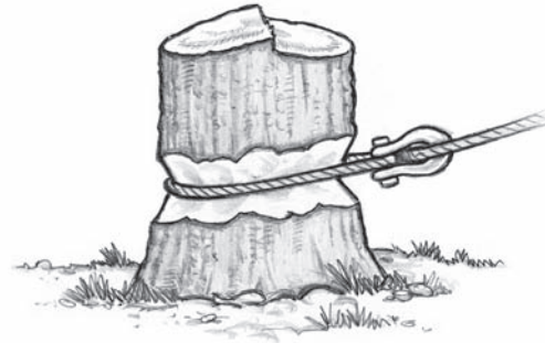
Correct notching: good depth, in lead
