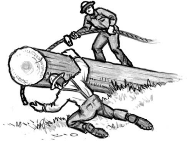
Proper setting of chokers: always go over the top of the log, except in rare circumstances.
