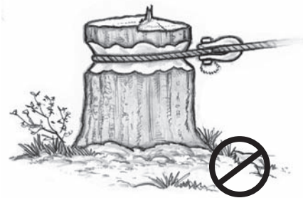
Improper notching: too close to top
