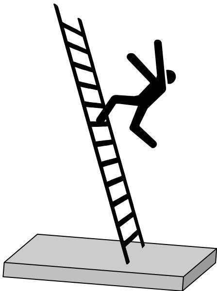
**Most falls involve portable ladders that move, tilt or shift while the worker is climbing or descending.**
