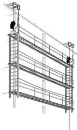
multilevel suspended scaffold
