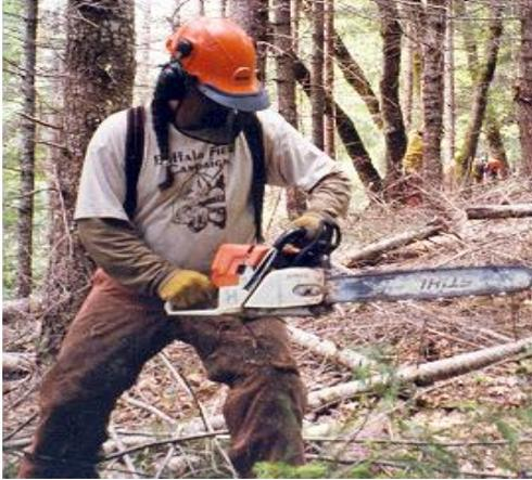
1. Avoid awkward positions. Reposition your body to maintain stability and control of the saw.
