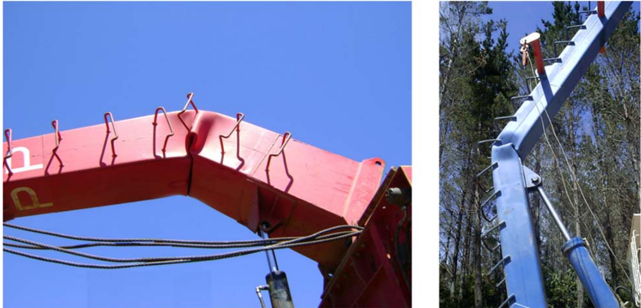
Figure 2. Tower lateral “buckling” due to excessive compressive forces. Source: Augusto Kahler. Operacion con cables en torres de madereo.
