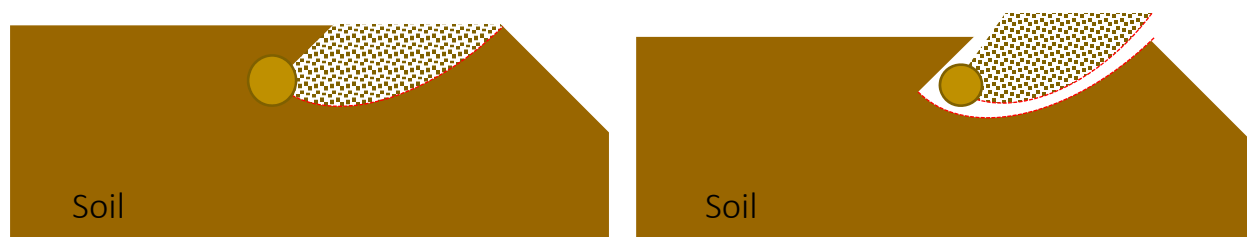
Figure 3. Logarithmic spiral soil rupture pattern before and after pullout.
