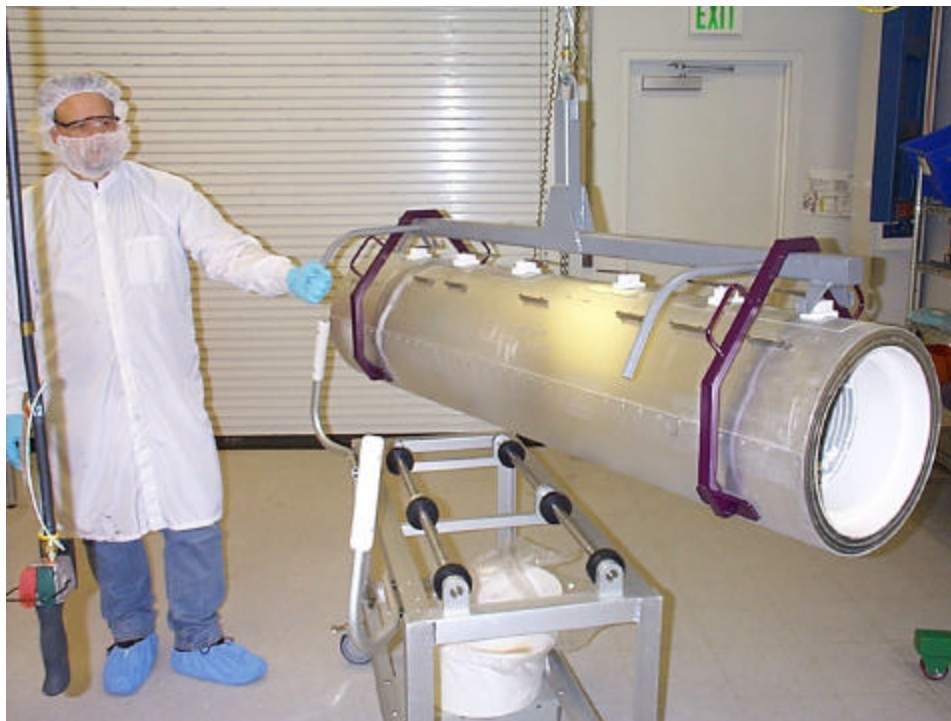
Heater core being lifted onto cart by preclean crane
