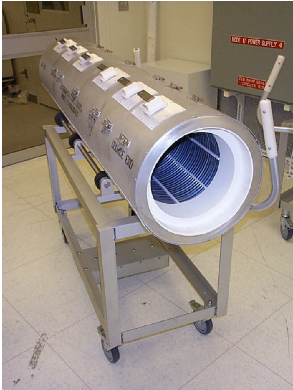
Heater core on dedicated cart. Note rollers which allow the core to be rotated for preparation work and handles to guide cart from both ends. Counter weight (bottom center) adds stability to the cart.
