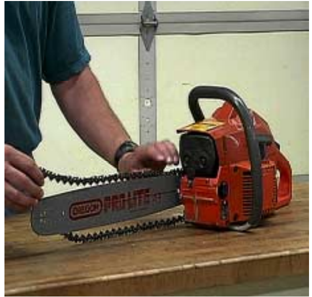
Saw chain being placed on a laminated chain saw guide bar
