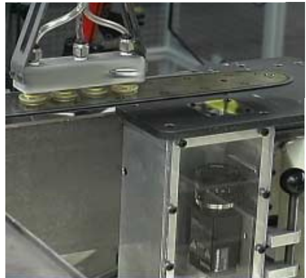
Tooling-hole of bar positioned over vision camera.
