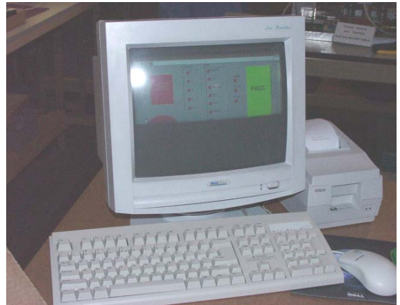
8. The computer gives a pass or fail message. If the control fails, a print out lists what the failure is.
