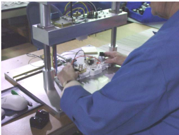
1. The test process starts by placing the control in the fixture.
