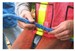
29. Bunching (compression) of bury section to facilitate sliding the fid forward.
