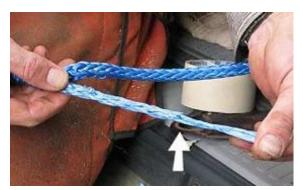
35. Removal of fid and tape from the tail end. Option to remove 3 more strands (at the halfway point of the 6 strand section) and further taper the end of the buried tail (12 to 6 to 3 strands at the end).
