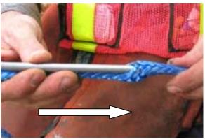
24. Insertion of fid point into opening of rope, created by in-line compression of the rope. Insert the fid into the center of the rope, while being careful not to hook any strands.
