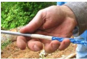
22. Fid is secured to the tapered tail. To aid in burying the tail, tape edges smooth to keep the fid and rope contour.
