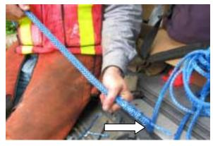
37. Tail of the buried 3 fid lengths about to be fully drawn into 3-1/2 fid length bury section to complete the eye.
