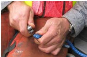
10. Knife blade is inserted under the entire marked strand and a cut is made.
