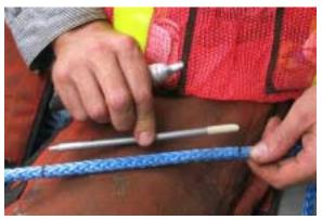
5. Marking off a fid length (or desired length) which will form the loop section of the eye splice.
