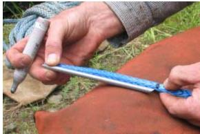
2. The first of three fid lengths is marked on the tail which will be buried for the eye splice.
