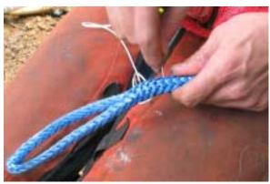
41. Continue the lock-stitching through the rope for 3 loops created on opposite sides of the rope.
