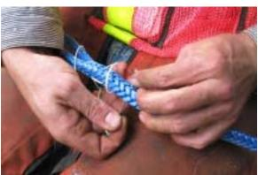
42. Rotate the needle direction 90 degrees and lock-stitch 3 loops on each side of the rope back towards the eye.
