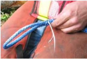
44. Final lock-stitch is finished to bring the end of the twine out the same position as initial entry point.
