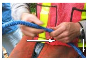
28. Continuation of sliding fid and buried rope toward the 3-1/2 fid (exit) mark. As the tail proceeds into bury section, it is best to grip the tail above the fid when stroking cover of bury section towards the eye. This should prevent pulling the taper end out of the fid (and having to start over).
