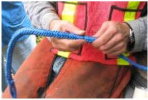
30. Take care not to pull the taped end of the rope off the fid when stroking cover near tapered end. Otherwise grip the rope above tapered end to keep taped attachment intact.
