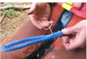
40. Lock-stitching the buried tail section with braided nylon twine and yarn needle. THIS IS NOT A STRENGTH ELEMENT. It prevents the manual removal of the buried tail section.
