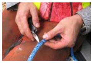
9. Initial cut of one strand of a marked pair in the first fid length of tail to be buried. Note black ink spot on marked pairs.
