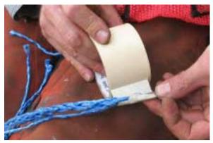
21. Securing the tapered tail to the fid with tape. Masking tape (2-inch wide) is sufficient for small diameter ropes, otherwise use duct tape.
