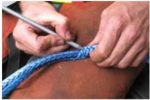
48. The end of the fid is used to push the knotted end of twine into the center.
