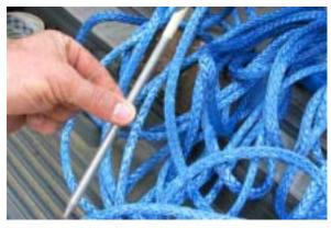
1. A splicing fid (aluminum needle) sized for the rope diameter to be spliced. The fid length for this 3/8-inch diameter rope is 8 inches.
