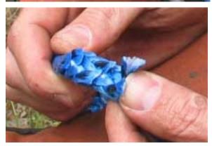
11. Profile of rope with some of the 6 marked strands cut. These strands are ready to be removed.
