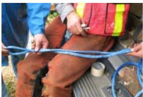
6. Marking off 3-1/2 fid lengths from the end of the loop section. The 3 fid or desired length tail will be buried into the center of this section to form the splice.
