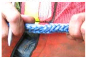
49. The exterior cover strands are moved into position over the knot for protection.
