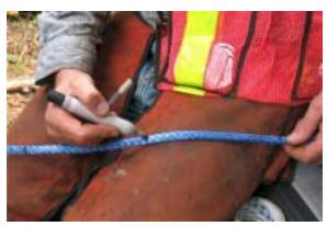
4. Marking off the second and third fid lengths on the tail which will be buried.
