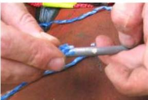
20. Insertion of the tapered tail into the fid.
