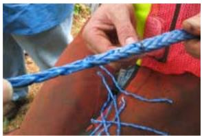
18. Tapered tail, tight weave, 6 strands. Note strands are cut such that the cut end does not project out from the rope, which aids in burying the tail.
