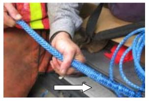
36. Stroking the cover bury section, from the formed eye, towards the exposed tail. This will allow the tail to be drawn into the center and covered.
