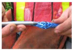
23. Creation of opening for pointed end of fid by inline compression of rope (see photo 7). The entry point is 3 fids plus desired loop length from end of tail (previously marked).
