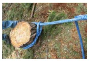
51. Prior to use, load (pull-on) the line to 10 percent of it's breaking strength to remove the construction stretch in the rope and eye splice.
