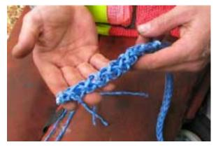
15. Fid length tail of rope, showing 6 remaining strands in loose weave.
