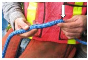
31. Fid exiting center of rope at or beyond the 3-1/2 fid (exit) mark. The mark in this photo is at the end of the left index finger, with fid point just at the left thumb.
