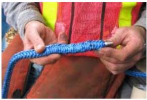
32. Continuation of fid removal from the bury section. Again, take care not to pull the tapered end off the taped end of the fid.
