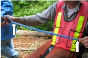
38. Completed eye splice. Length of buried rope extends from the end of the eye to the pinched rope section in the splicer's left hand.
