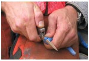
12. Continuation of cutting of the 6 marked strands (3 marked pairs).
