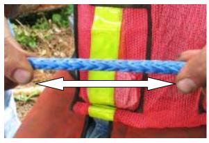
8. In-line extension of the 12 strand braided rope to show rope elongation and re-establishment of the rope cross section after compression.
