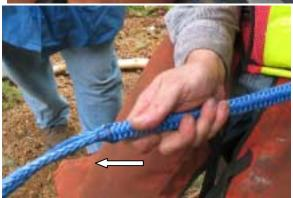
34. Stroking the cover bury section and pulling of the buried end to bring the loop into the desired size for the eye.
