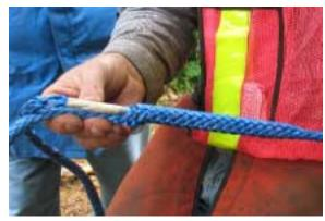
25. Stepwise insertion of the fid and attached tapered end into the 3-1/2 fid length bury section.
