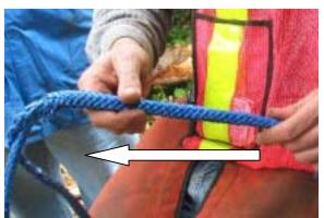
27. Stroke exterior of the rope bury section towards the eye while maintaining a grip on the pointed end of the fid and/or buried rope. This extends the bury section over the buried tail.
