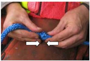
26. Compression of the rope to open the center for the next stepwise forward progression of the fid.
