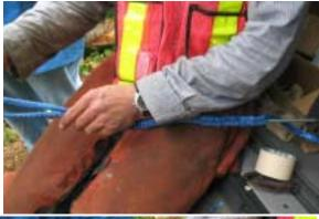
33. Alignment of the loop section of the rope to create a smooth transition of the buried section at the eye formation point (fid entry point).
