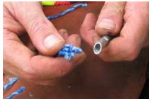
19. End of tapered tail, compressed for insertion into the end of the fid.
