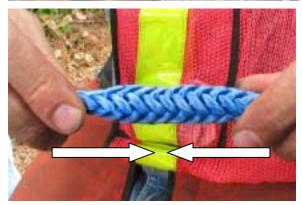
7. In-line compression of the 12 strand rope to open the rope center for fid insertion. Note length shortens, thus the need for 3-1/2 fids to bury the 3 fid tail.
