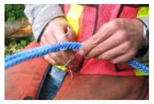
43. Approaching the end of the lock-stitch. Note the tail of the twine is extending out from the initial entry point.
