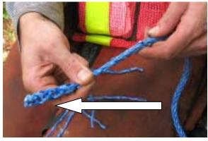
17. Stroke loose weave tail from first fid mark to end of tail to establish the taper section.
