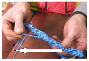
13. Removal of one of the 6 cut strands by pulling from the cut end away from the tail of the rope.
