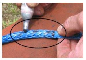
3. Marking off 3 alternate pairs of strands from the first fid mark. The marked pairs will be cut and removed to taper the end of the rope. Note spots on the strands near the end of the marker pen.
