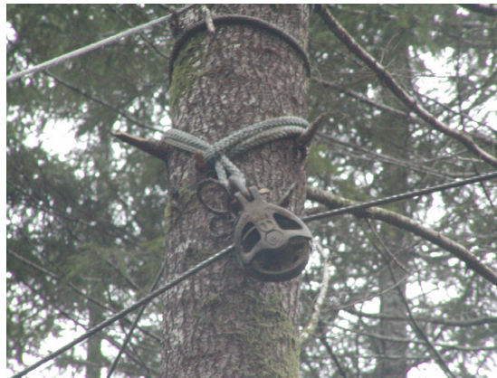
Figure R7. Synthetic rope in an endless loop configuration used as a tree strap.
