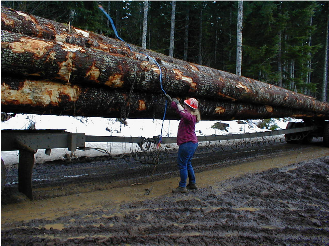
Figure R13. A female driver throws an additional synthetic rope wrapper on an off-highway load that requires two 7/16" diameter wrappers.
