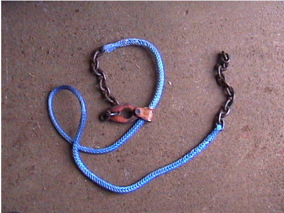
Figure R25. Prototype synthetic choker using Farmi winch line keyhole slider as a choker bell and chain ends for connecting to log and to winch line slider.
