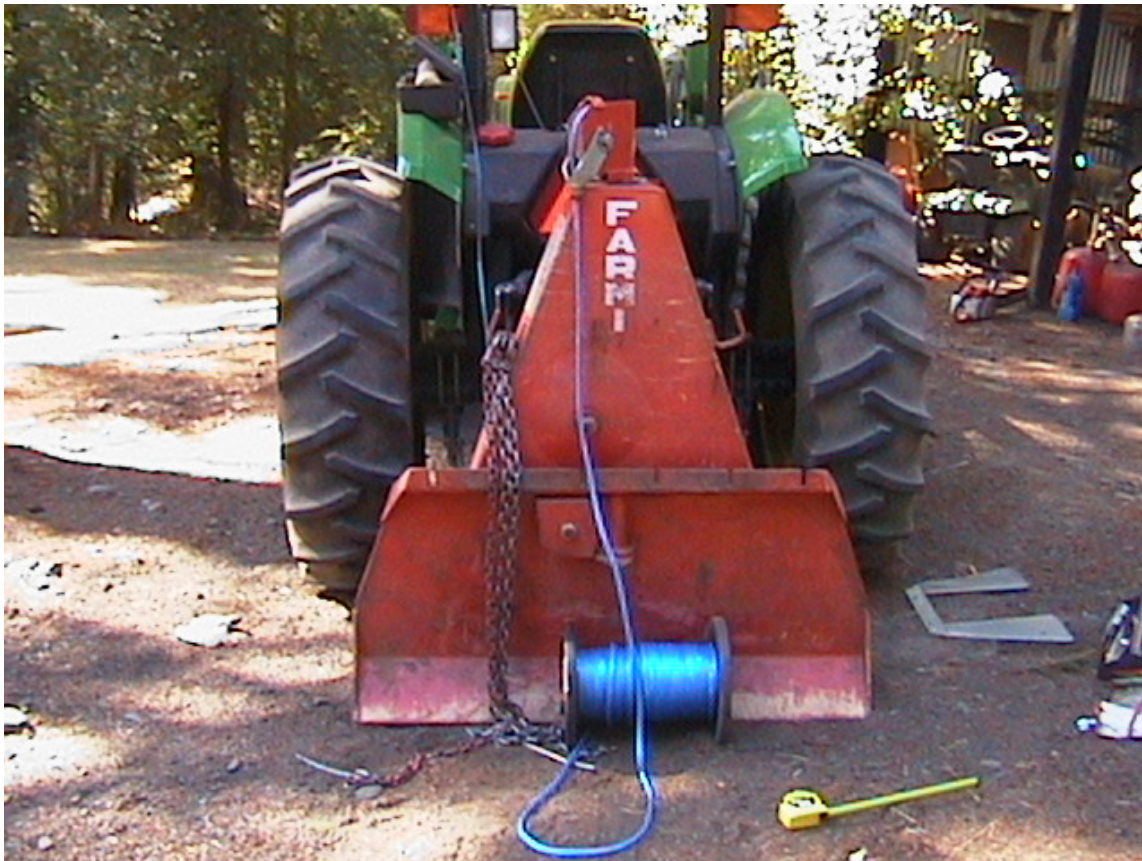
Figure R24. Farmi winch system mounted on farm tractor and powered by power take-off (PTO) drive. Chain chokers shown were initially trialed until replaced with synthetic rope based chokers.
