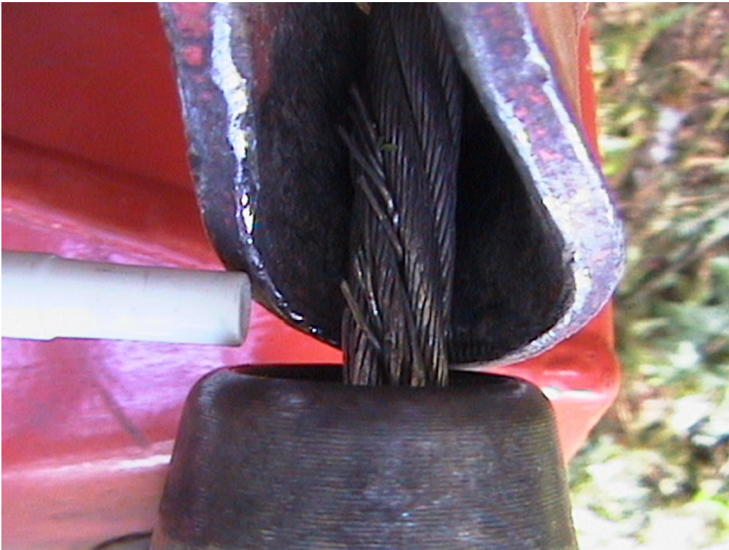
Figure R10. Line showing broken wire or “jagger” that will inflict lacerations and puncture wounds during handling of steel wire rope.
