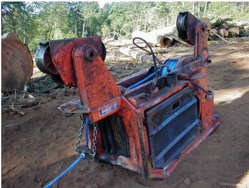
Figure R27. Synthetic rope installed on slackpulling carriage. Carriage design does not incorporate a line slackpulling device, but rather depends on the stiffness of steel to “push” the line of the drum. A minimal tension applied to the synthetic rope during the slack phase prevents backspooling of the synthetic rope due to its lack of stiffness.
