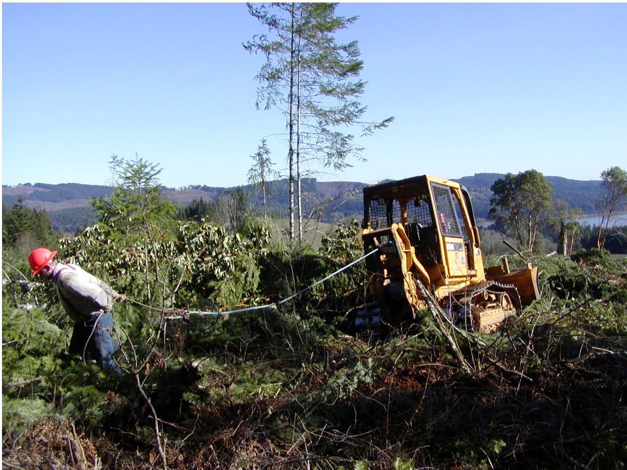
Figure R23. Operator pulling synthetic winch line to a log. Note two pear ring sliders staged along winch line for logs to be hooked.
