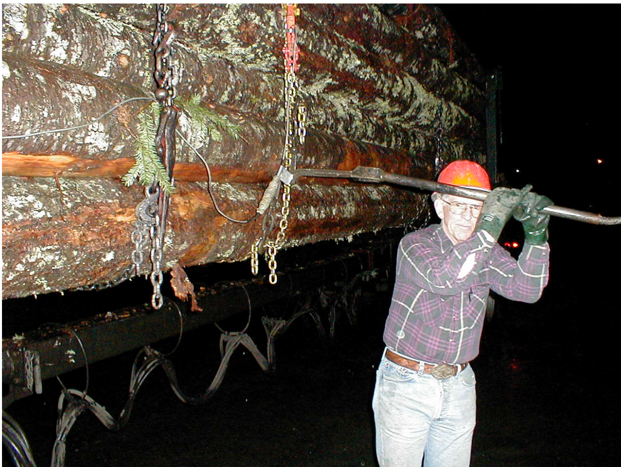
Figure R5 shows driver attaching load binder to steel wrapper on the load. Note use of the binder handle extension or “cheater bar” and tension monitoring device wiring
