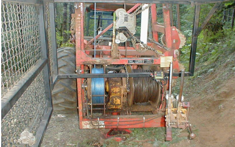
Figure R28. Synthetic mainline on Koller K300 yarder winch set. Drum spooled 1300 feet of 3/8-inch diameter synthetic rope compared to 1150 feet of steel wire rope capacity.
