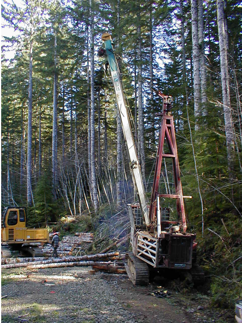
Figure R19. Diamond 210 yarder operation utilizing synthetic rope for static line applications of rigging straps, intermediate support guylines and jack support line.
