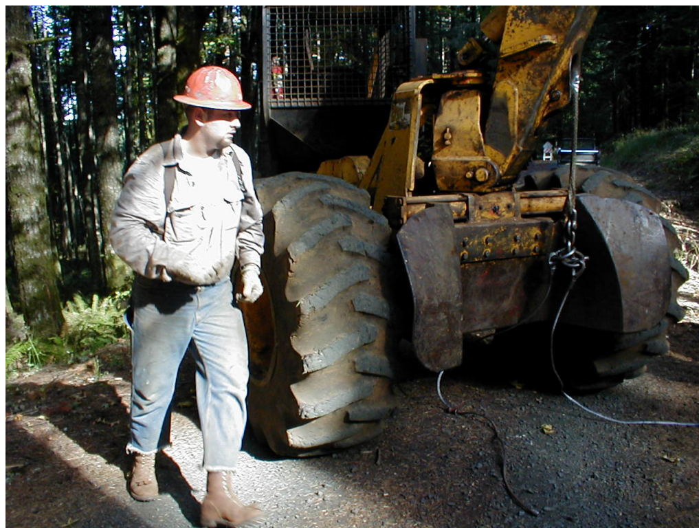
Figure R3 shows skidder operator moving to take the winchline and chokers to the logs.
