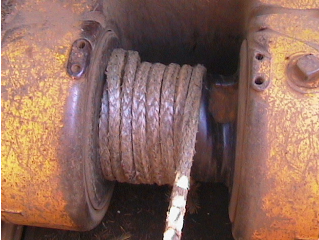
Figure 33. Spooling the winch line on the drum under tension by pulling the machine with the winch.
