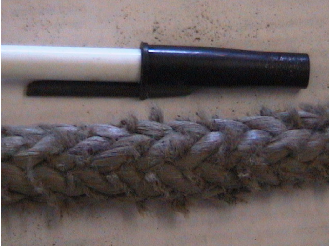
Figure 46. Section of a 3/8-inch diameter ASB synthetic rope wrapper with accumulation of cut filaments.
