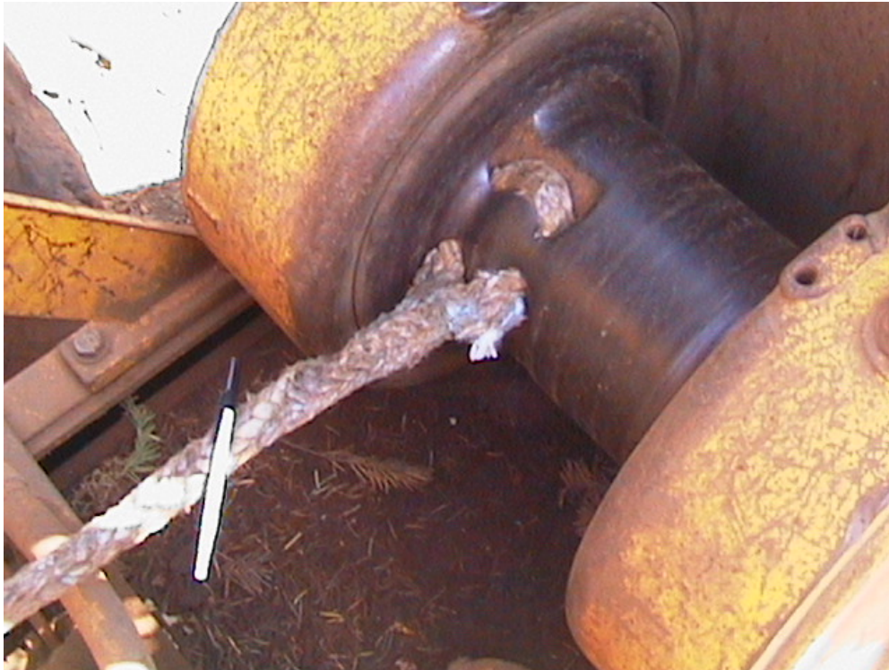
Figure 32. Short buried eye splice to connect the synthetic winch line to the skidder drum.
