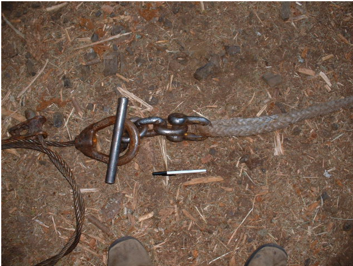
Figure 35. Working end of winch line termination is a function of hardware. Shown is ring and T-bar toggle set-up commonly used for presetting chokers with quick off-on of empty and set chokers. Connection of steel hardware to synthetic rope is created with the simple Buried eye splice.
