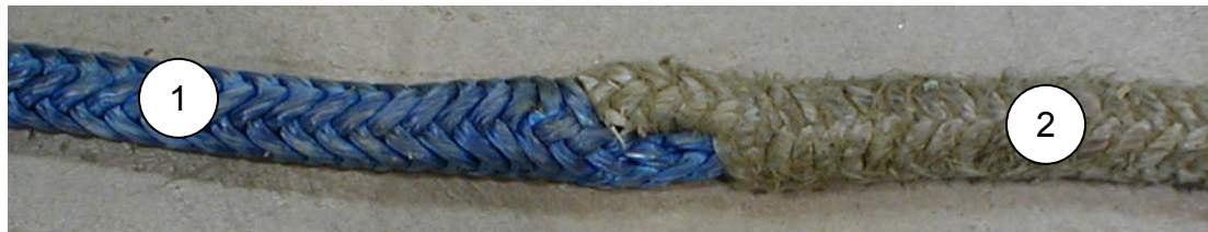
Figure 8. Finished long splice
