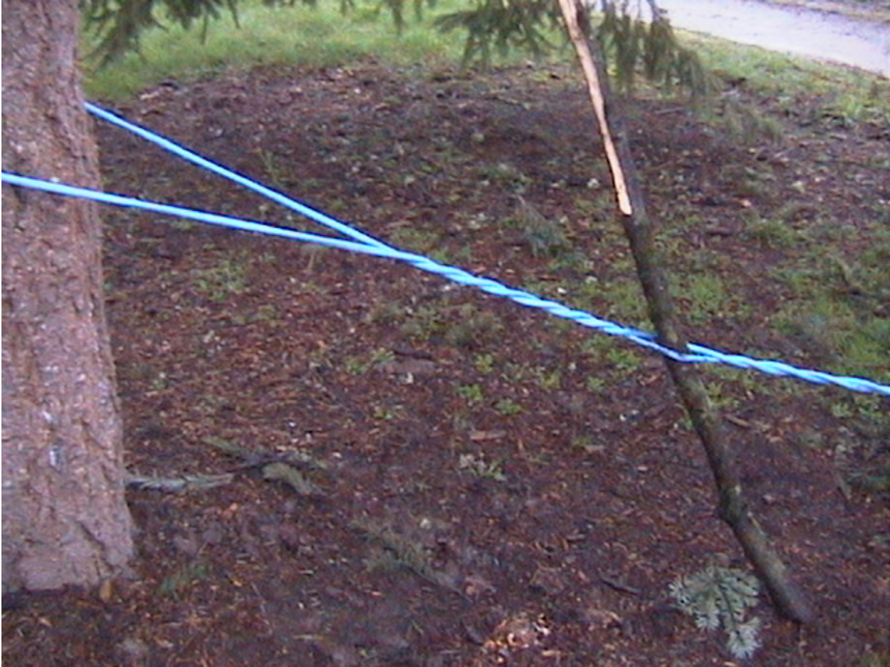
Figure 20. Twister shown made with 3/8 – inch diameter synthetic rope.
