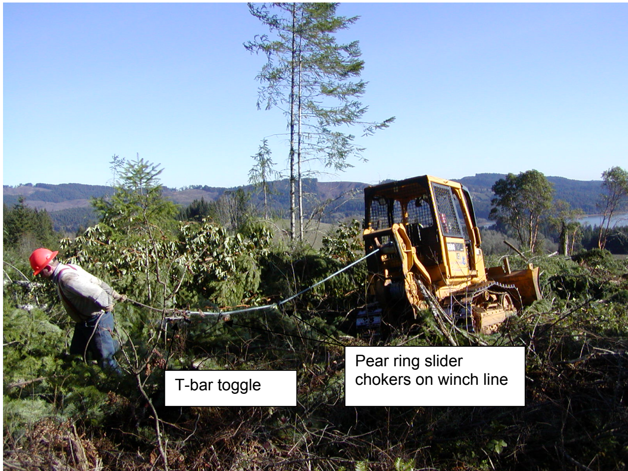
Figure 36. Operator pulling synthetic rope off of crawler tractor winch. Pear-ring choker slid up against “T-bar toggle” and two more chokers on winch line.
