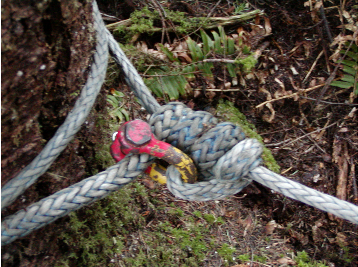
Figure 24. Close up of shackle connected to buried eye splice (yellow end) and locked back on the tail of the eye splice. Extra wraps around secondary section of guyline (to right of photo) used take up short length of slack (slack length insufficient to complete an additional wrap). If eye and shackle had just reached the guyline (to right of photo), no extra wraps would be required – just shackle the eye onto the secondary guyline section.
