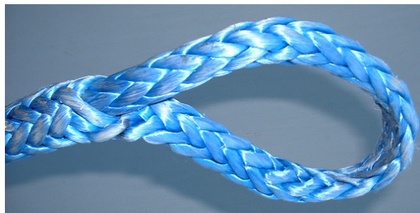
Figure 4. Buried eye splice
