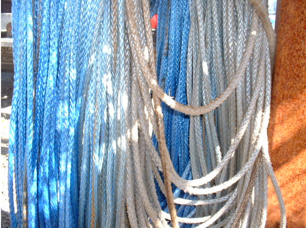
Figure 43. Gradation of color with normal use. Shown is the 3/8-inch diameter ASB synthetic rope mainline for a Koller K300 yarder.
