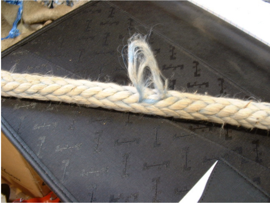
Figure 49. Pulled yarn (collection of filaments) from a single strand of a 12 strand ASB synthetic rope. Pulled yarns and strands should be re-threaded to prevent snagging and further malformation of the rope structure during operation.
