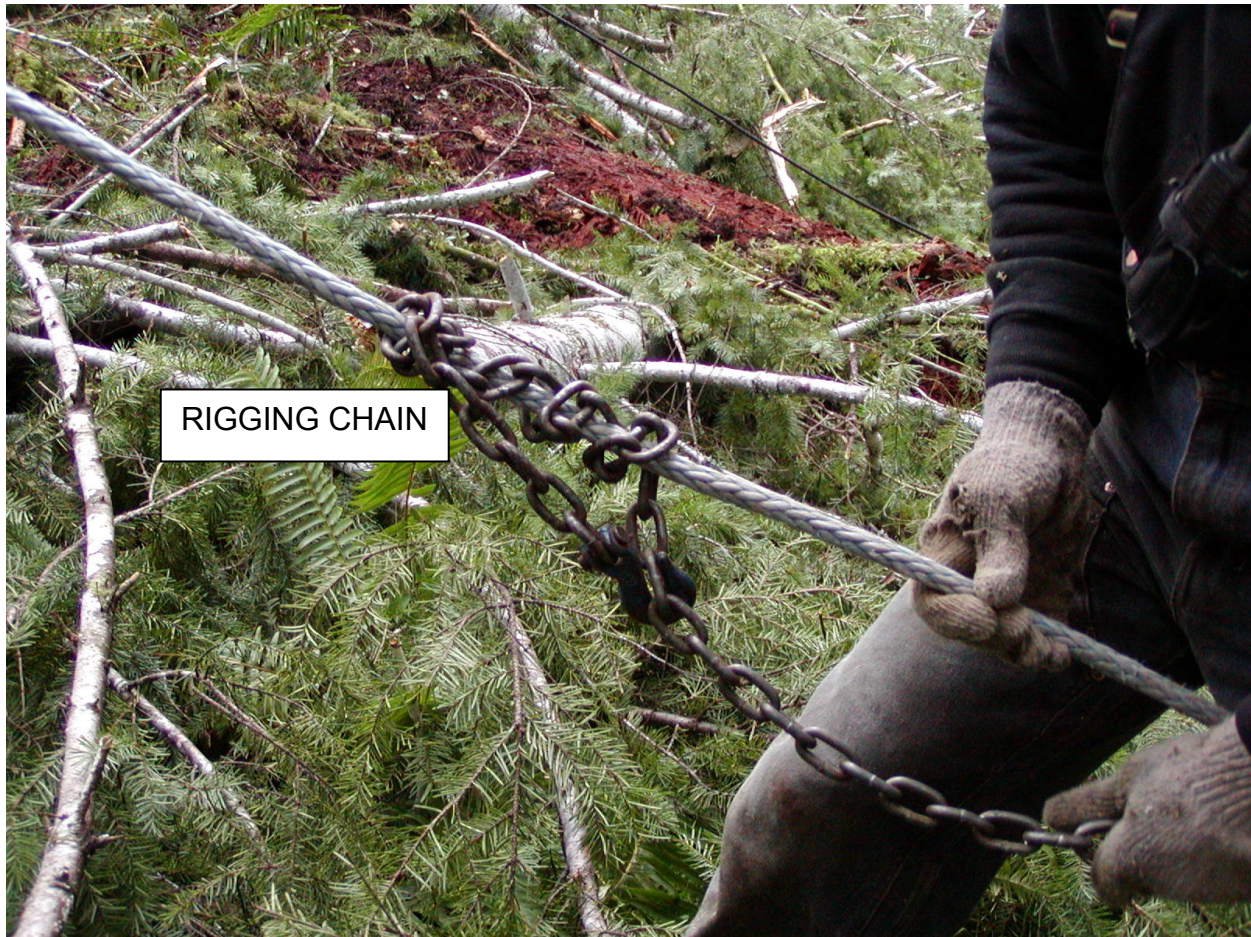
Figure 19. Rigging chain wrapped around synthetic rope guyline for tensioning with come-along. Note the use of a grab hook and the direction of wrap to prevent rigging chain from sliding along the synthetic rope.
