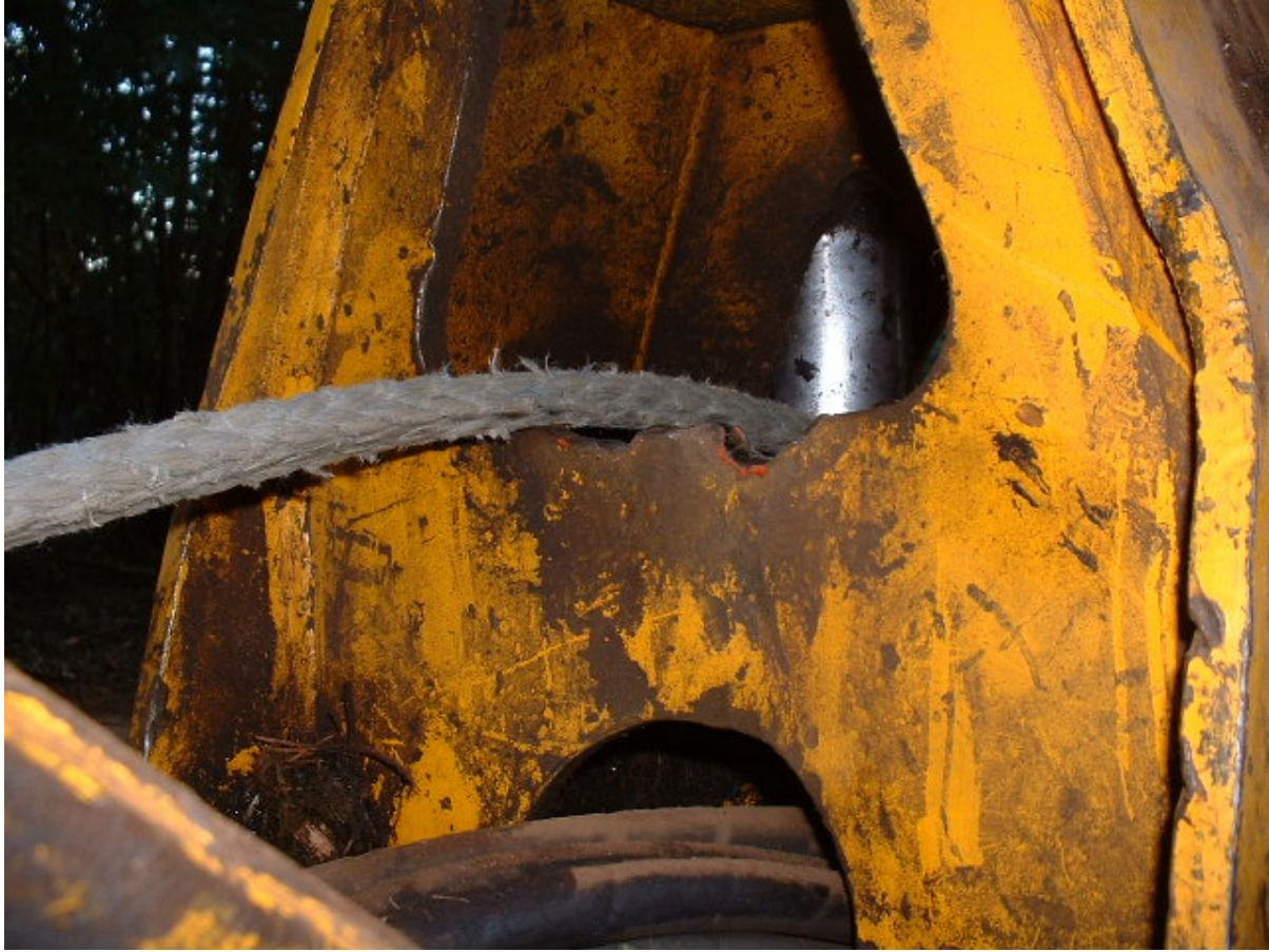
Figure 51. Grooves shown are cut in ½-inch steel plate by steel wire rope under improper operation of fairlead arch. Abrasive surfaces such as this must be dressed smoothly prior to use of synthetics. Synthetic rope will not stand the abuses that steel wire rope will. Continued operation in this mode will create undue shortening of operational life of synthetic rope due to fraying of fibers and strands, with a resultant reduction in rope strength.
