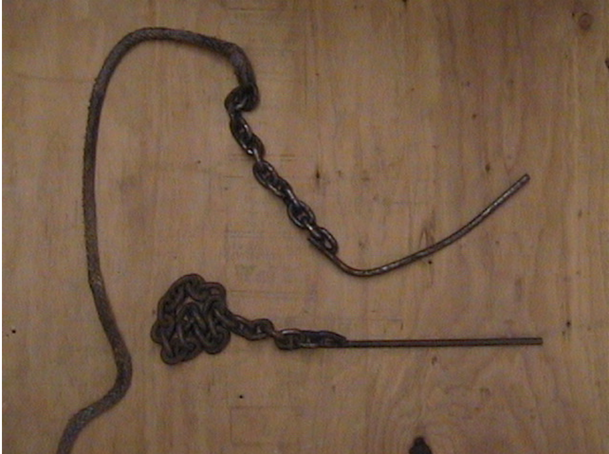
Figure 41. A short length of 5/16-inch diameter steel rod was added to the end of one chain to facilitate feeding the synthetic choker under a log and feeding the chain into the Farmi slider (see Fig. 40). The rod was heated, fed through the chain, looped closed and welded shut. With use, the rod tends to form a curve that aids in feeding it through the choker hole.
