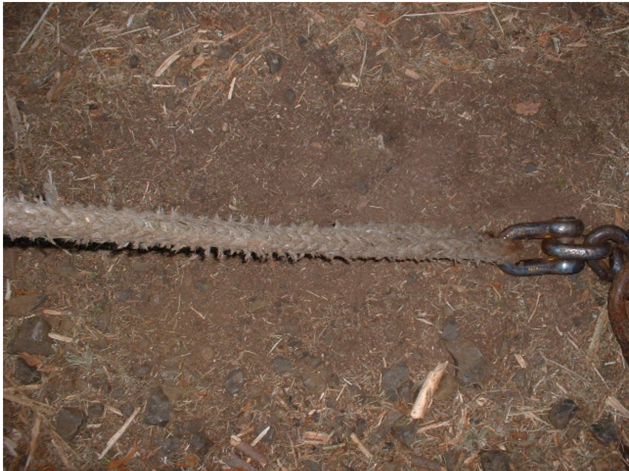
Figure 44. Rope appearance. Fuzzed filaments and tufts (local accumulation of fuzzed filaments) on the end of a skidder winch line. Continuous abrasion by the ring sliders created this condition. Rope failures have occurred near the buried tail of this eye splice, but not in the splice section itself. This is considered an acceptable wear condition for this application as the skidder winch line. Synthetic winch lines which experience cut strands that are not taken out of service or repaired (spliced) should be
