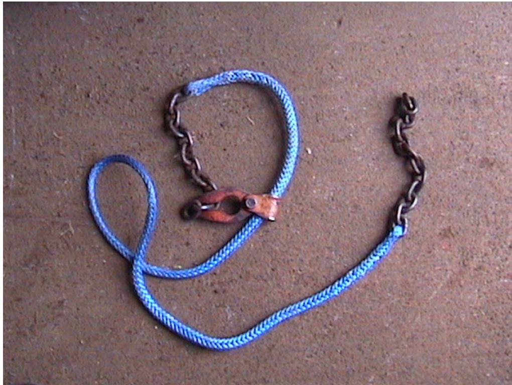
Figure 40. Prototype synthetic choker made with 3/8-inch diameter ASB synthetic rope. A Farmi winch line keyhole slider is used as a choker bell with a chain end to act as the nubbin. The other chain end is for connecting the hooked log to the winch line slider.
