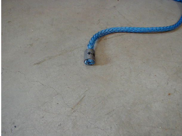
Figure 30. Packed butt splice nubbin used as a breakaway attachment to the drum.
