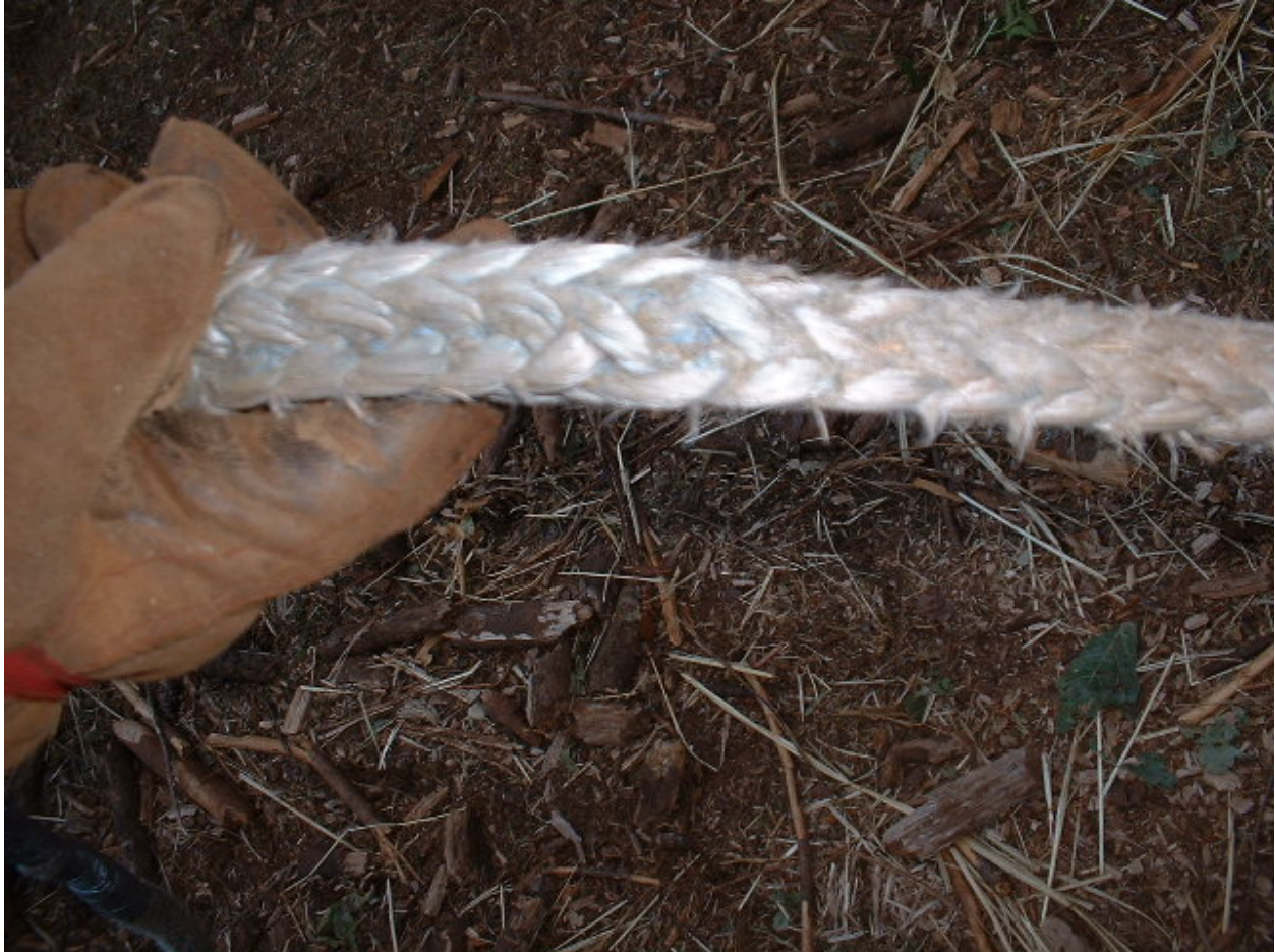
Figure 45. Section of skidder winch line from Figure 44 located away from the working end. Note reduction in quantity and quality of tufts. Also note residual blue coating on the internal portion of the strands.
