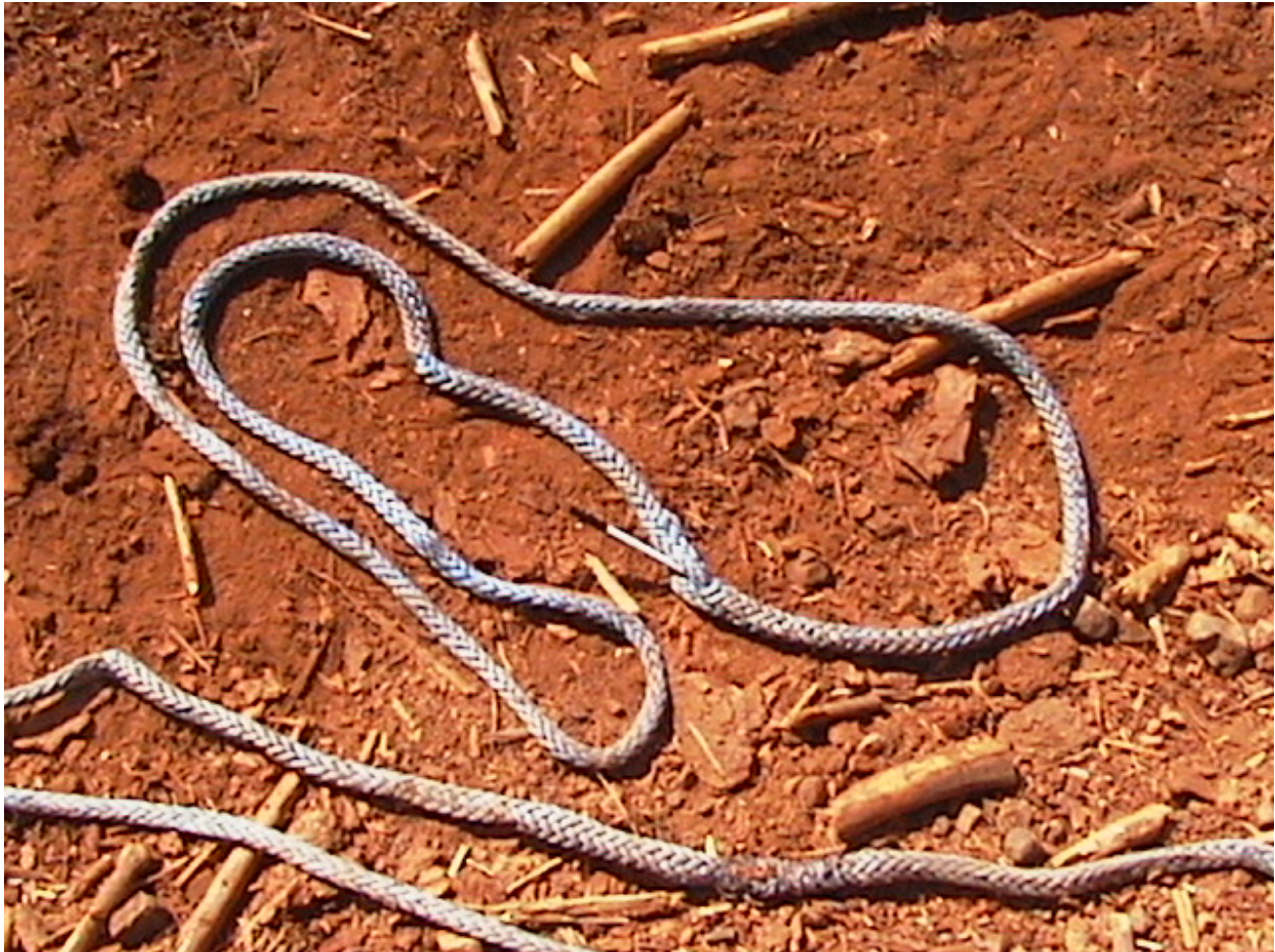
Figure 3. Loop strap of synthetic rope with pen showing end for end (long) splice connection.
