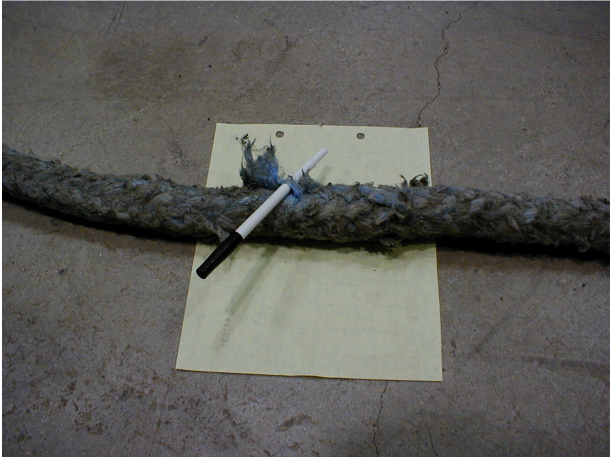
Figure 47. Severe abrasion in a section of 7/8-inch diameter ASB synthetic winch line. Pen is inserted underneath the intact remnants of a strand. Manufacturer's recommendation is to retire a rope or cut and re-splice the remaining rope when 2 or more adjacent strands are cut.
