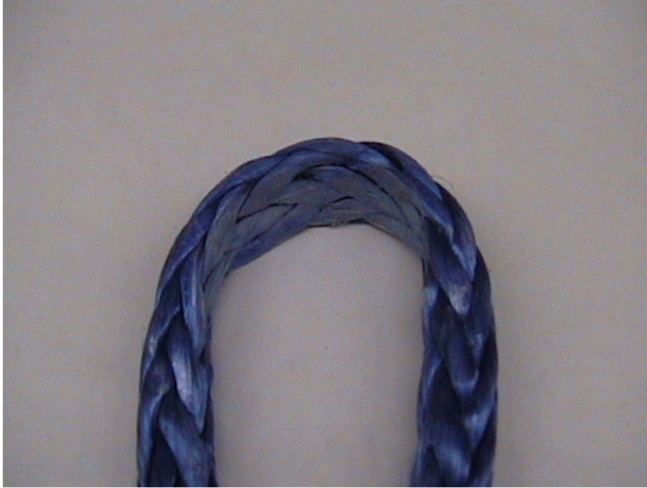
Figure 50. Fiber set due to compressive loading around the barrel of a drum winch. Note slightly glazed appearance. Flexing of the rope should eliminate this appearance and allow for continued use of the rope.
