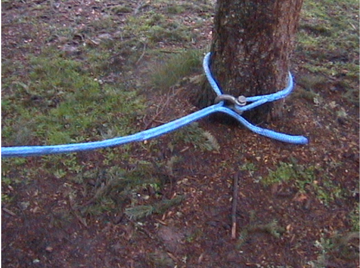
Figure 17. Adjustable guyline extension (slack) using “whoopie sling” technique with synthetic rope.
