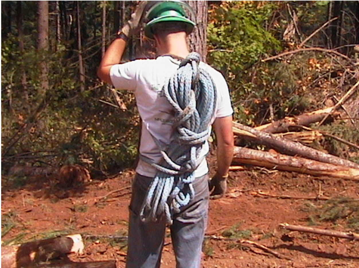
Figure 42. Synthetic rope guyline coiled for ease of carrying (not possible with steel guylines). This technique is adapted from rock climbing.
