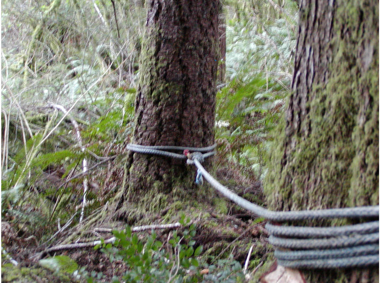
Figure 23. Guyline end secured to second tree (or stump), shackle end connected to eye splice (buried eye splice) and back onto extra length of guyline reaching between initial anchor (in foreground) and terminal anchor.
