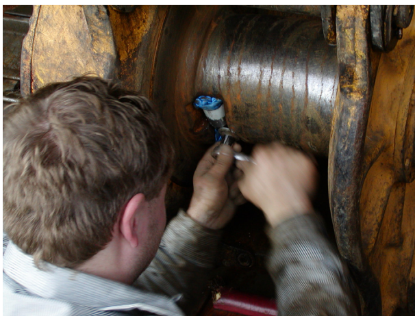
Figure 31. Attaching the packed butt splice nubbin end connector to the drum barrel.
