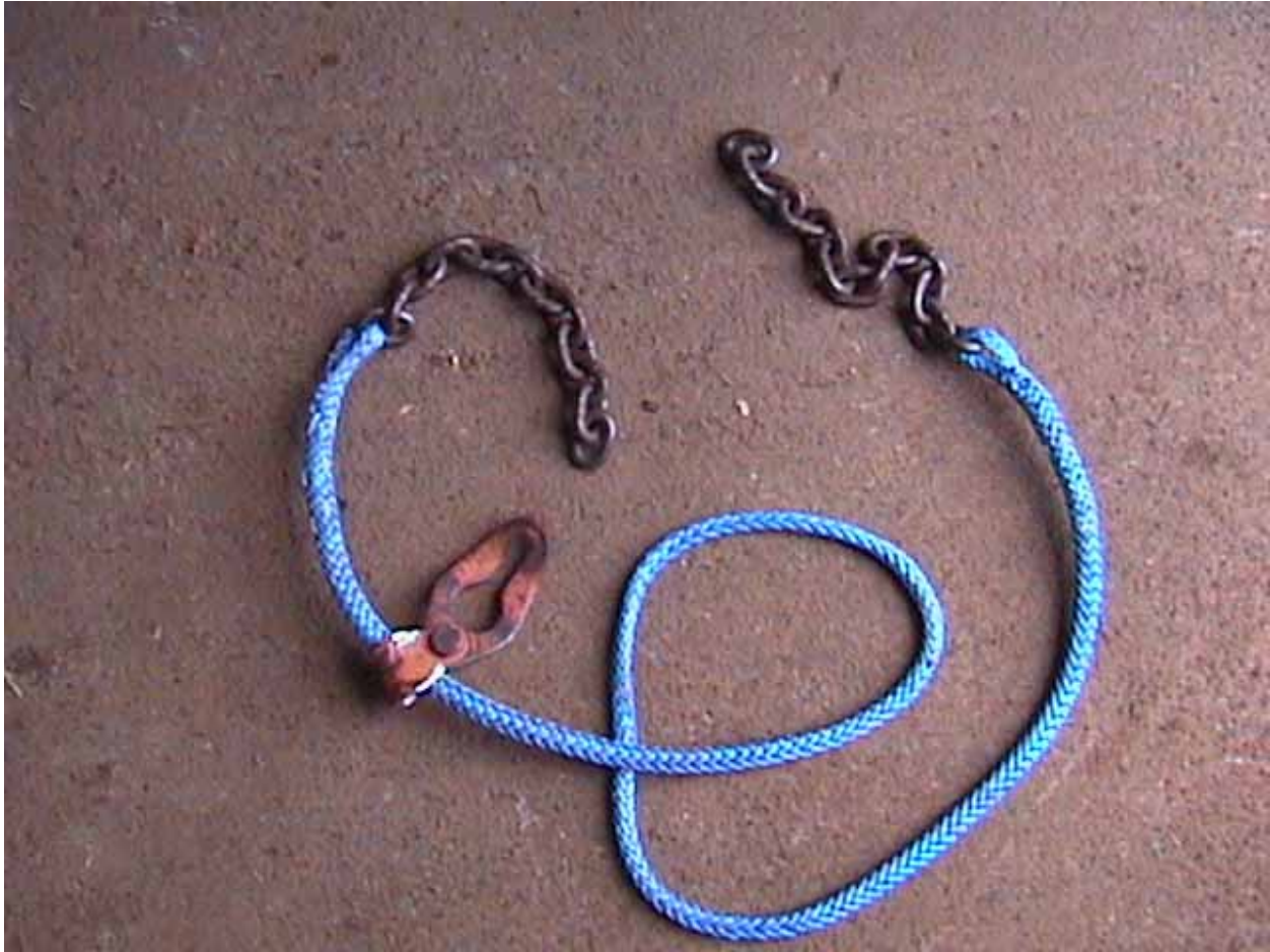
Figure 2. Prototype log choker using chain, synthetic rope, and a Farmi slider hook for a choker bell to replace chain choker.
