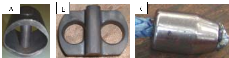
Figure 2. End connections with hardware: A) Pinned nubbin B) Knuckle link C) Pressed nubbin
