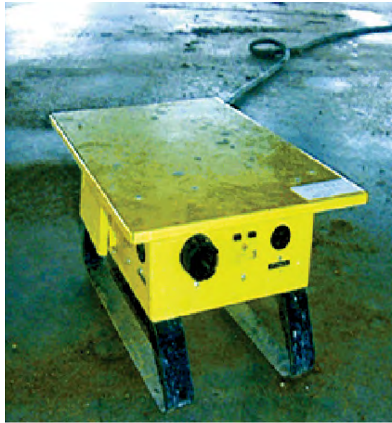
Typical "Spider box" supplies GFCI-protected receptacle for use on construction sites.
