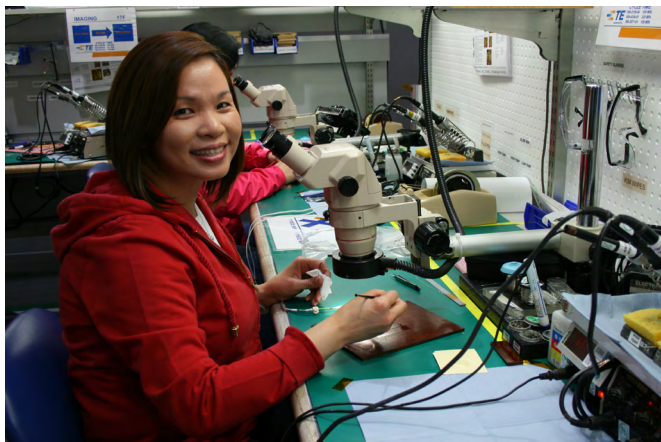
Left: Dung Nguyen solders fine wire onto a printed circuit board.
