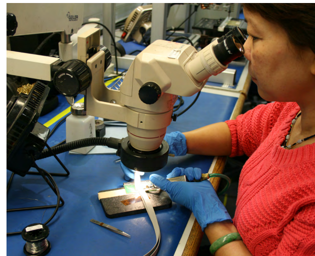
Hoa Tran solders conductors to a printed circuit board at TE Connectivity.
