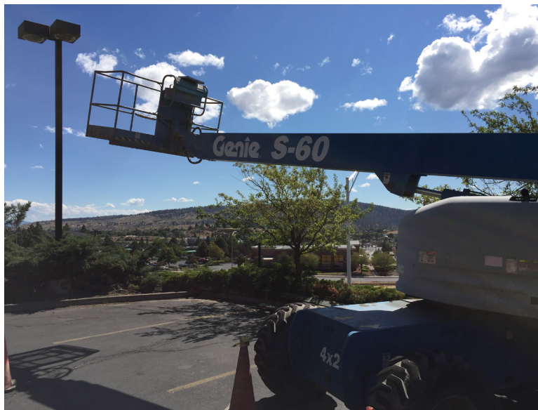
The 26,060-pound Genie S-60 lift; the operating instructions on Genie S-60 control console were illegible.
