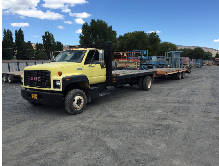
The truck and trailer; the lift's weight exceeded the trailer's carrying capacity.
