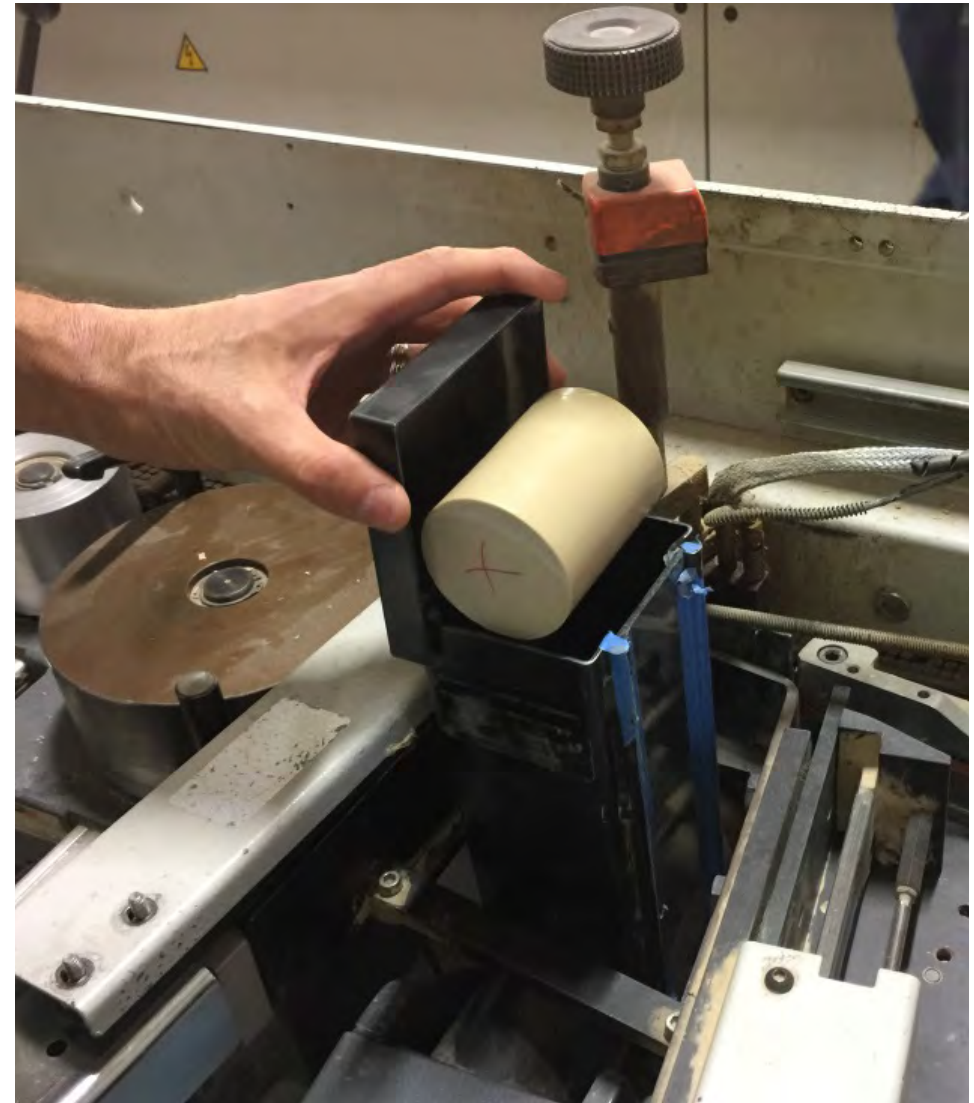
A glue puck being loaded into the hopper of the edge banding machine.
