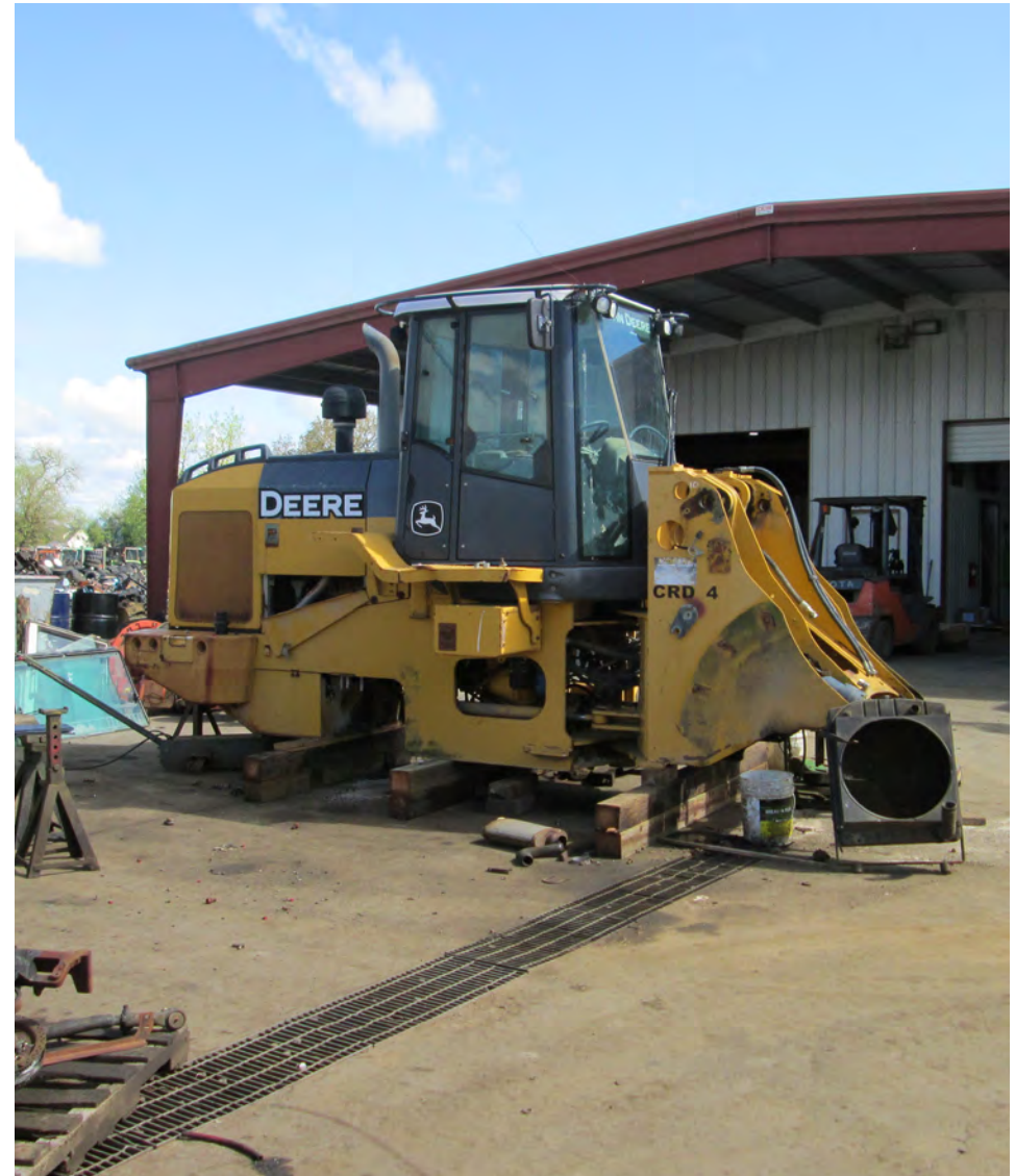
The John Deere 624J front-end loader after the front and rear axles had been removed.
