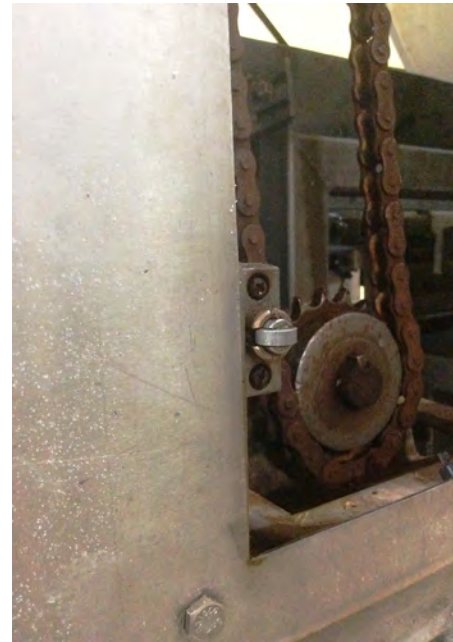
Close-up of the safety door switch and the gap between the chains. The sprocket rotates counter-clockwise.
