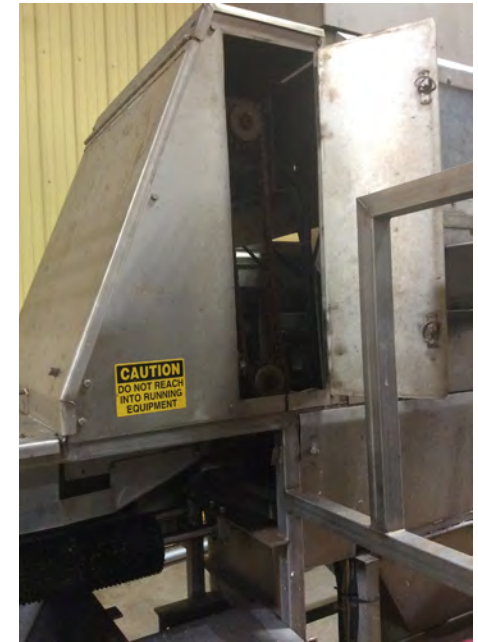
The open safety door on the onion peeling machine. Note the warning sign to the left of the opening.
