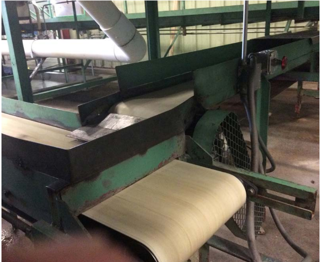
The corner where the two conveyers met. The worker was standing on the inside of corner facing the conveyor belt on the right side of the photo. Note: The employer installed the emergency start-stop switch on the right after the incident.
