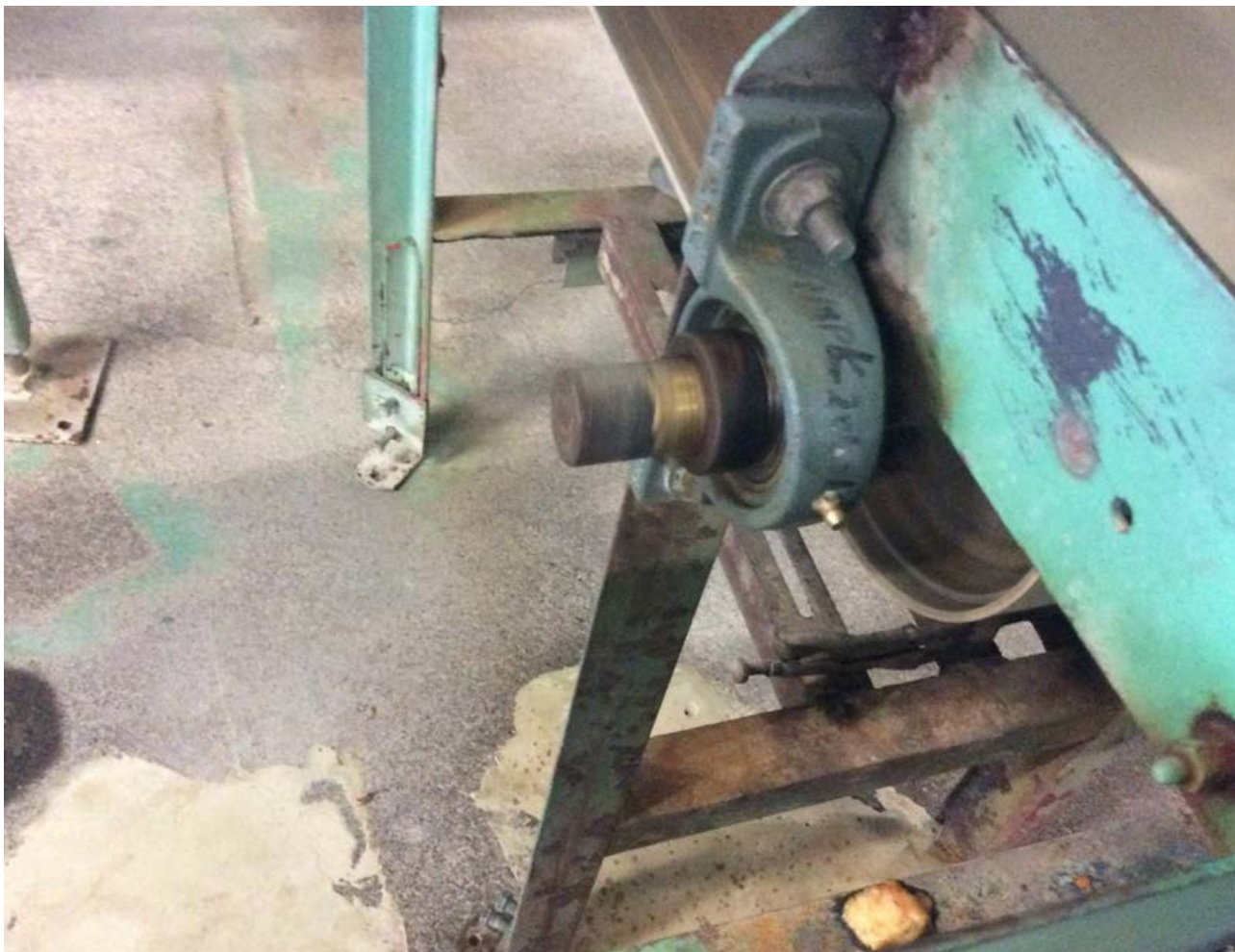
The worker's rain jacket was caught in this exposed pulley shaft.
